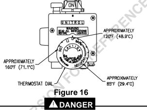
Hotter water increases the risk of scald injury. Scalding may occur within five (5) seconds at a temperature setting of  $135^{\circ}$  F ( $57^{\circ}$  C). To protect against hot water injury, install an ASSE approved mixing valve in the water system. This valve will reduce point of discharge temperature by mixing cold and hot water in branch water lines. A licensed plumbing professional or local plumbing authority should be consulted.
